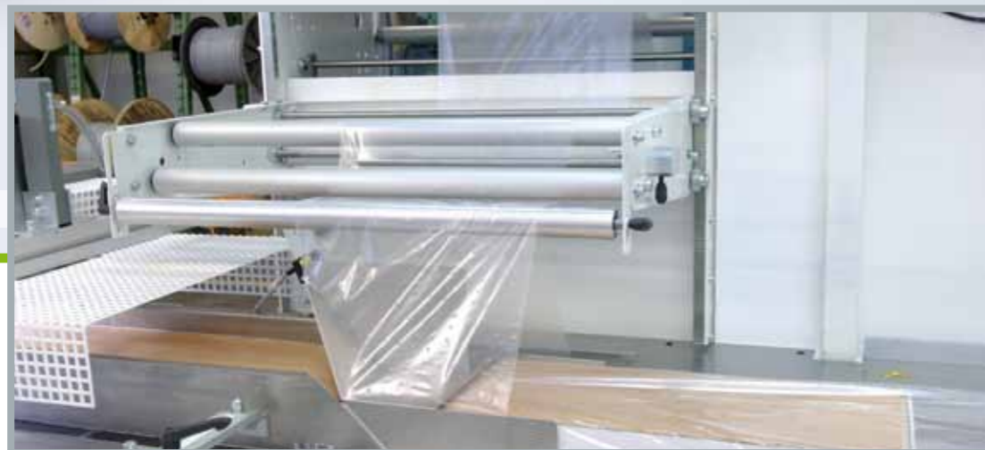
servo X: Laminate packaging with solid forming shoulder
